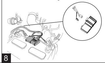
Connect power and ground for controller to battery, Red to positive and Black to the negative lead. Route harness legs down over wheel wells toward motor linkages, long leg across front and over to driver side. Secure all loose sections of the harness with cable ties.
