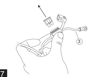
Secure controller to vehicle wire loom beside battery (on passenger side) and connect both Power Step wire harness connectors to connectors on controller. Secure locking tabs on connectors.
