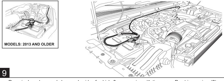
Run wire legs down and along underside of vehicle floor, securing with tie wraps. Run trigger wires (2) on Drivers side through grommet as shown below.
