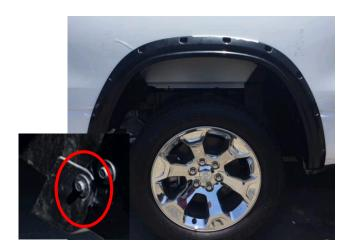
**STEP 10:** Position Fender Flare so that the top (3) slots engage with the raised heads of the grey screw plugs. Using philips head screws, <u>loosely install</u> flare into postion. Using previously removed hex screws, <u>loosely install</u> remaining (5) screws at location (A). Ensure cut out in flare fits around factory mud spat. When satisfied, <u>completely secure</u> the (8) locations.
