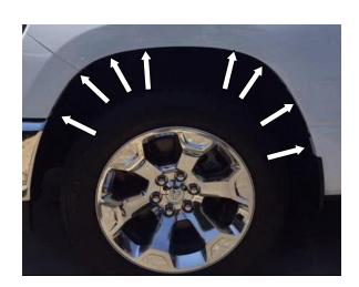
**STEP 5:** Hold Fender Flare towards vehicle in the position of best fit. Note the (8) slots in the flare that correspond with factory installed hex screws in the wheel arch. Remove these (8) and retain for later re-installation.
