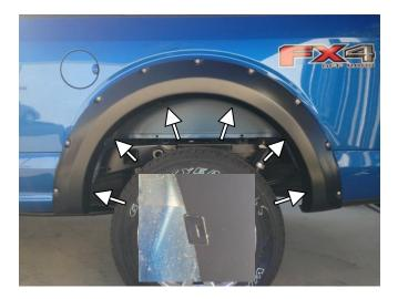
**STEP 16:** Place the Fender Flare onto the vehicle and fit into the correct position following the contours of the body. Use 6 of the U-style clips to secure the Fender Flare to the body. Make sure the barb in the clip securely attaches in the slot on the Fender Flare.
