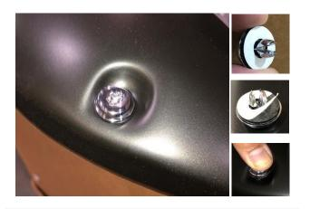
**STEP 11:** Attach the extruded plastic bolts. Peel back white tape liner from the bottom side of the extruded plastic bolt and press until it snaps into place. Ensure inside of Fender Flares where the rubber seal is attached is clean, using the alcohol wipes provided. Wipe away any residue with a dry clean cloth.
