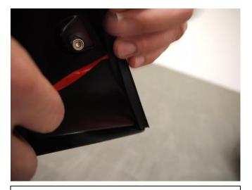
**STEP 13:** Pulling at right angles to the extrusion, remove the liner from the extrusion in small portions and apply thumb pressure to ensure that it adheres to the Fender Flares.
