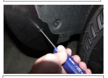
**STEP 9:** Re-install factory screw in the mudguard using #15 Torx head screwdriver through the slot in the Fender Flare.
