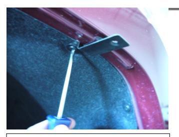
**STEP 7:** Apply clear tape to the inside edge of the fender wheel arch in front of positions **A** and **B** (step 5) over mastic sealant. Install the large brackets in positions **A** and **B** (step 5) aligning the slot in the bracket with the vacant holes from the factory screws in the vehicle wheel arch. Ensure clips are positioned over the clear tape. Reinstall the factory screws in location **A** and **B** using a #15 Torx head screwdriver.
