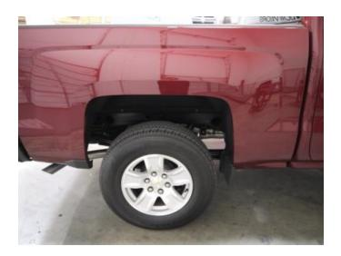
**STEP 14:** Clean the body areas where the Fender Flares will make contact. Ensure fenders are dry prior to install.
