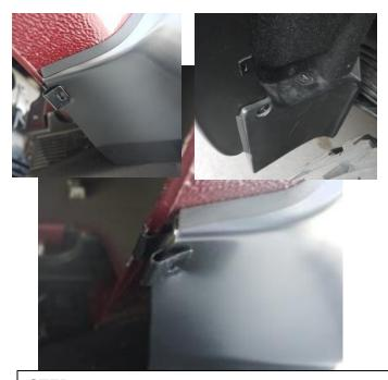
**STEP 17:** Slide the top edge of rear front mudguard cut out behind the factory mudguard. Install the E shape clip so that the clip slides over the inner sheet metal lip and is in line with the slot in the underside of Fender Flare. To secure the clip to Fender Flare apply inward tension on Fender Flare to the vehicle fender when installing the E clip, position the clip so that the barb in the clip locates in the slot of the Fender Flare.
