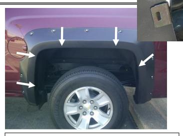
**STEP 16:** To secure the Fender Flare to the body, apply upward tension on Fender Flare to the vehicle fender when installing the black metal clips. Slide the clips over the Fender Flare and the inner wheel arch lip in the five locations shown. Position the clip so that the barb in the clip locates in the slot of the Fender Flare.
