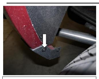
**STEP 15:** Using #15 Torx head screwdriver remove upper screw from the rear factory mudguard. Maintain screws for re-install.
