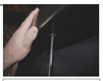
**STEP 8:** Place Fender Flare on the vehicle into the position of best fit so the slots in position **A** and **B** are over the holes in the front end of large clips. Ensure bottom rear slot in Fender Flare is located over the vacate hole in the factory mudguard. Apply upward tension on Fender Flare to the vehicle fender when Installing the screws and washers provided into the clips in position **A** and **B** using a Philips head screwdriver.
