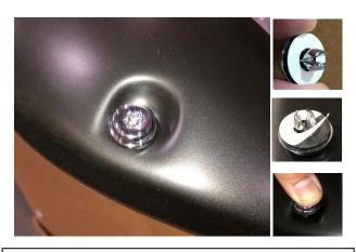
**STEP 11:** Attach the extruded plastic bolts. Peel back white tape liner from the bottom side of the extruded plastic bolt and press until it snaps into place. Ensure inside of Fender Flares where the rubber seal is attached is clean, using the alcohol wipes provided. Wipe away any residue with a dry clean cloth.
