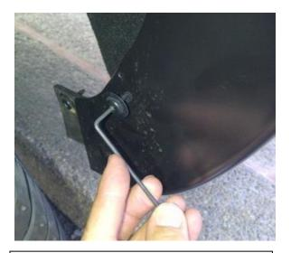
**STEP 18:** Using #15 Torx head screwdriver reinstall the upper screw from the rear factory mudguard through the slot in the Fender Flare. Ensure all fixing points are tight and secure and that the rubber seal is flush neatly against the vehicle body.
