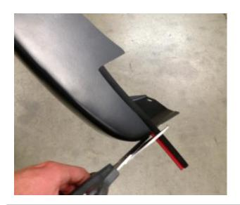
**STEP 13:** Attach rubber seal to the bottom front corner of Fender Flares. Peel back 1" of the adhesive backing and position on the Fender Flare. Attach the seal to the Fender Flare, ensure pressure is used to secure rubber seal to Fender Flare edge. Trim excess rubber seal and discard.
