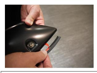
**STEP 12:** Attach the included rubber seal to the Fender Flares. Peel back 2" of the adhesive backing and position on the Fender Flare. Attach the seal to the Fender Flare, peeling back a few inches at a time. Ensure pressure is used to secure rubber seal to Fender Flare edge. Attach rubber seal along all areas the Fender Flare will make contact with the vehicle body. Trim excess rubber seal.
