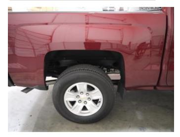
**STEP 13:** Clean the body areas where the Fender Flares will make contact. Ensure fenders are dry prior to install.
