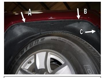
**STEP 5:** Place Fender Flare on the vehicle into the position of best fit. Note where the slots in Fender Flare at positions **A** , **B** and **C** align with the existing screws in the vehicle wheel arch. Remove Fender Flare. Remove the existing vehicle screws in location **A**, **B** and **C** using #15 Torx head screwdriver. Maintain screws for re-install.
