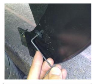
**STEP 16:** Using #15 Torx head screwdriver reinstall the upper screw from the rear factory mudguard through the slot in the Fender Flare. Ensure all fixing points are tight and secure and that the rubber seal is flush neatly against the vehicle body.
