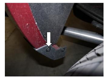
**STEP 14:** Using #15 Torx head screwdriver remove upper screw from the rear factory mudguard. Maintain screws for re-install.
