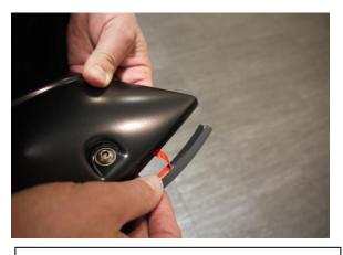
**STEP 11:** Attach the included rubber seal to the Fender Flares. Peel back 2" of the adhesive backing and position on the Fender Flare. Attach the seal to the Fender Flare, peeling back a few inches at a time. Ensure pressure is used to secure rubber seal to Fender Flare edge. Attach rubber seal along all areas the Fender Flare will make contact with the vehicle body.
