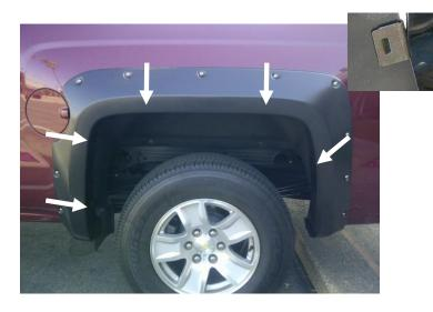
**STEP 15:** To secure the Fender Flare to the body, apply upward tension on Fender Flare to the vehicle fender when installing the black metal clips. Slide the clips over the Fender Flare and the inner wheel arch lip in the five locations shown. Position the clip so that the barb in the clip locates in the slot of the Fender Flare.
