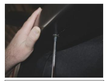
**STEP 8:** Place Fender Flare on the vehicle into the position of best fit so the slots in position **A**, **B** and **C** are over the holes in the front end of large clips. Ensure bottom rear slot in Fender Flare is located over the vacate hole in the factory mudguard. Apply upward tension on Fender Flare to the vehicle fender when Installing the screws and washers provided into the clips in position **A**, **B** and **C** using a Philips head screwdriver.
