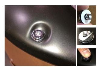
**STEP 10:** Attach the extruded plastic bolts. Peel back white tape liner from the bottom side of the extruded plastic bolt and press until it snaps into place. Ensure inside of Fender Flares where the rubber seal is attached is clean, using the alcohol wipes provided. Wipe away any residue with a dry clean cloth.
