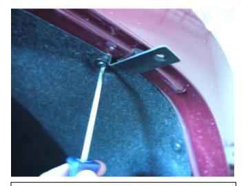
**STEP 7:** Apply clear tape to the inside edge of the fender wheel arch in front of positions **A**, **B** and **C** (step 5) over mastic sealant. Install the large brackets in positions **A**, **B** and **C** (step 5) aligning the slot in the bracket with the vacant holes from the factory screws in the vehicle wheel arch. Ensure clips are positioned over the clear tape. Re-install the factory screws in location **A**, **B** and **C** using a #15 Torx head screwdriver.
