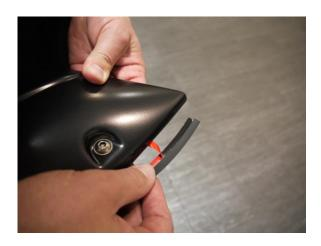
**STEP 2:** Attach the included gasket to the Fender Flares. Peel back 2" of the adhesive backing and position on the Fender Flare. Attach the gasket to the Fender Flare, peeling back a few inches at a time. Ensure pressure is used to secure gasket to Fender Flare edge. Attach gasket along all areas the Fender Flare will make contact with the vehicle body.
