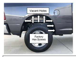
**STEP 9:** Hold Fender Flare towards vehicle in the position of best fit. Note (4) slots in Flare that correspond with factory installed hex screws, and the (3) that correspond with vacant holes in wheel arch. Remove (4) screws and retain for later reinstallation.
