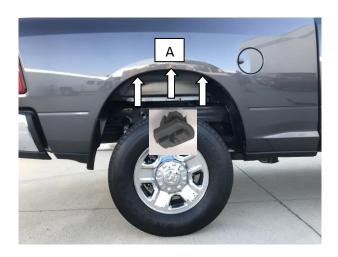
**STEP 10:** Insert grey screw plug into vacant holes at position (A) ensuring that the raised head of the screw plug runs parallel with vehicle body.
