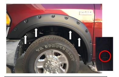
**STEP 6:** Using the previously removed hex head screws, <u>loosely install</u> flares beginning at the front of the flare working to rear. Ensure the cut-out shape fits around factory mud spat against vehicle surface. Ensure the previously removed one inch of tape liner from front and rear Fender Flares is on the outside of the rubber gasket. When satisfied with position, <u>completely secure</u> the (4) hex screws.
