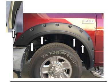
**STEP 5:** Hold Fender Flare towards vehicle in the position of best fit. Note the (4) slots in the flare that correspond with factory installed hex screws in the wheel arch. Remove factory hex screws and retain for later re-installation. Peel back one inch of tape liner for the rubber gasket each end of the Fender Flares then fold at 45 degrees outside of the Fender Flare. Remove one inch of tape liner from the rubber gasket that locates around the factory spat.
