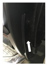
**STEP 12:** Starting at the front of the Fender Flare, carefully remove tape liner from rubber gasket a few inches at a time. Ensure rubber gasket is not tucking into flare and sits flush neatly against the fender body. Ensure all fixing points are tight and secure. Apply forward pressure to adhere the gasket along the edge of entire length of Fender Flare once gasket liner is removed. Repeat install steps for the opposite side of the Fender Flares.
