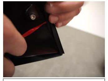
**STEP 3:** Pulling at right angles to the extrusion, remove the liner from the extrusion in small portions and apply thumb pressure to ensure that it adheres to the Fender Flares.
