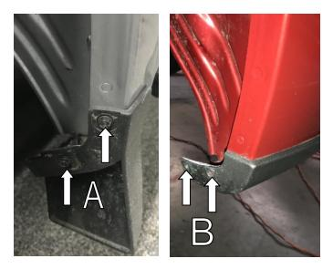
**STEP 12:** Remove the two 7mm factory wheel well spat bolts (A) and the two rear factory retainer clips (B), retain for installation of Fender Flares. Rentainer clips (B) will need to be removed using needle noise pliers.
