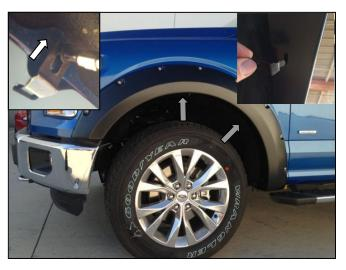
**STEP 8:** Place the Fender Flare onto the vehicle and fit into the correct position following the contours of the body. Use 2 of the retaining clips and 7.0mm bolts to secure the Fender Flare to the body. Make sure the clip securely engages the Fender Flare.
