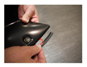
**STEP 2:** Attach the included rubber seal to the Fender Flares. Peel back 2" of the adhesive backing and position on the Fender Flare. Attach the seal to the Fender Flare, peeling back a few inches at a time. Ensure pressure is used to secure rubber seal to Fender Flare edge. Attach rubber seal along the top leading edge of the Fender Flare where it will make contact with the vehicle body.
