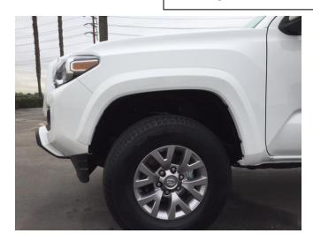
**STEP 1:** Clean the vehicle body areas with a mild soap and water solution, where the Fender Flares will make contact. Ensure fenders are dry prior to install.
