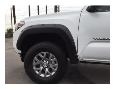
**STEP 9:** If necessary, make minor adjustments to the flares position to achieve the best fit for your vehicle and to ensure that the rubber seal is sitting flat against the painted vehicle surface. When satisfied fully tighten all (5) screw locations, in the above order in which they were just installed. Repeat install for opposite side.
