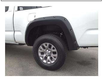
**STEP 16:** If necessary, make minor adjustments to the flares position to achieve the best fit for your vehicle and to ensure that the rubber seal is sitting flat against the painted vehicle surface. When satisfied fully tighten all screw locations, in the above order in which they were just installed. Repeat install for opposite side.
