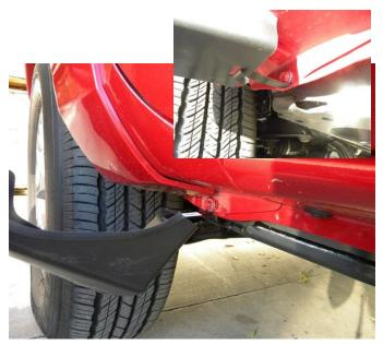
**STEP 6:** Begin installation by engaging the hook end of the clip into the slot in the bottom of the Fender Flare and begin rotating the Fender Flare vertically up to its position of best fit.
