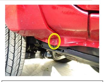
**STEP 4:** Again using a 10mm socket, remove the screw from the body sheet metal join referenced in STEP 5 as Special Note area "A" and retain for later re-installation.
