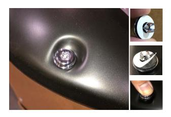
**STEP 1:** Attach the extruded plastic bolts. Peel back white tape liner from the bottom side of the extruded plastic bolt and press until it snaps into place. Ensure inside of Fender Flares where the rubber seal is attached is clean, using the alcohol wipes provided. Wipe away any residue with a dry clean cloth.
