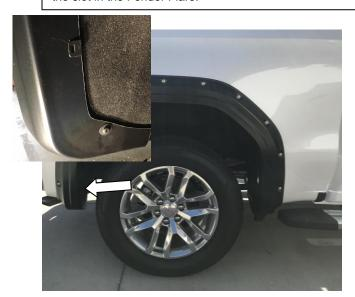
**STEP 15:** Using #15 Torx head screwdriver reinstall the previously removed factory mudguard screws at the upper screw locations through the slots in the front of the Fender Flare at the noted location.
