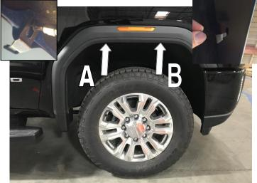
**STEP 6:** Using #15 Torx screwdriver remove factory screws at location **A** and **B**. Place Fender Flare on the vehicle into the position of best fit. Note where the slots in Fender Flare at positions **A**, **B** and vehicle wheel arch are located. Install the large clips to the inner wheel arch by sliding clips into the Fender Flare slots, ensure notch in the clip locates securely into the Fender Flare slot. Re-install the factory screws through the hole in the clips to the wheel arch
