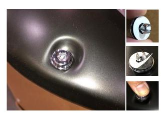
**STEP 9:** Attach the extruded plastic bolts. Peel back white tape liner from the bottom side of the extruded plastic bolt and press until it snaps into place. Ensure inside of Fender Flares where the rubber seal is attached is clean, using the alcohol wipes provided. Wipe away any residue with a dry clean cloth.
