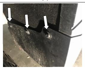
**STEP 12:** Using #15 Torx head screwdriver remove the three screws from the rear factory mud guard in the rear wheel arch. Fender flares require the rear mud guards to be removed, maintain screws for re-install if required.
