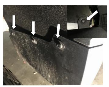
**STEP 5:** Using #15 Torx head screwdriver remove the three factory screws from the front mudguards and one underside screw location, maintain screws for re-install. Fender flares require the mud guards to be removed. Retain factory mudguards for later use if required.
