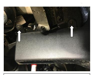
**STEP 13:** Using #15 Torx head screwdriver remove the upper and lower screws from the underside of the rear factory spat in the rear wheel arch. Maintain screws for reinstall. On the front spat using #15 Torx head screwdriver remove the lower screw from the underside that aligns with the slot in the Fender Flare.
