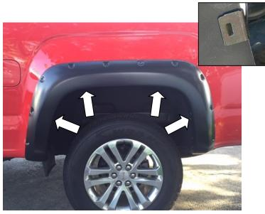
**STEP 13:** Install the provided U shape metal clips at the (4) remaining slot locations in the Fender Flare. Ensure that positive pressure is applied on the Fender Flare to the vehicle fender when installing clips. Slide the clips over the Fender Flare and the inner lip of the wheel arch molding ensuring that the barb in the clip locates in the slot of the Fender Flare.
