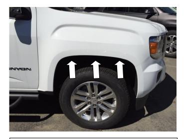
**STEP 5:** Place Fender Flare on the vehicle into the position of best fit. Note where (3) slots in Fender Flare correspond with (3) existing screws in the vehicle wheel arch molding. Remove Fender Flare. Remove the existing vehicle screws in location as shown #15 Torx head screwdriver. Maintain screws for re-install.
