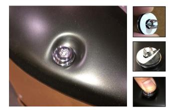
**STEP 1:** Attach the extruded plastic bolts. Peel back white tape liner from the bottom side of the extruded plastic bolt and press until it snaps into place. Ensure inside of Fender Flares where the rubber seal is attached is clean, using the alcohol wipes provided. Wipe away any residue with a dry clean cloth.
