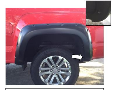
**STEP 14:** Using #15 Torx head screwdriver, re-install the previously removed srcew through the bottom rear slot in Fender Flare and factory deflector. Ensure all fixing points are tight and secure and that the rubber seal is flush neatly against the vehicle body and factory deflector.
