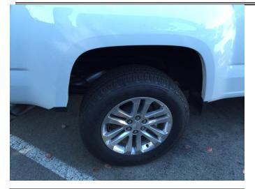
**STEP 10:** Clean the body area where the Fender Flares will make contact. Ensure fenders are dry prior to install.
