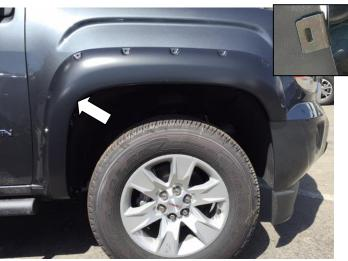
**STEP 8:** Install the provided U shape metal clip at the (1) remaining slot location in the Fender Flare. Ensure that positive pressure is applied on the Fender Flare to the vehicle fender when installing clips. Slide the clip over the Fender Flare and the inner lip of the wheel arch molding ensuring that the barb in the clip locates in the slot of the Fender Flare.
