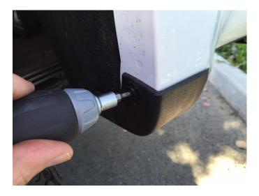
**STEP 6:** Using a #15 Torx head screwdriver remove bottom rear wheel arch molding screw. Maintain screws for re-install.
