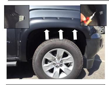
**STEP 7:** Place the Fender Flare onto the vehicle and fit into the correct position following the contours of the body. Use 3 of the retaining clips and previously removed factory screws to secure the Fender Flare to the body using #15 Torx head screwdriver. Make sure the clip securely engages the slots in Fender Flare.
