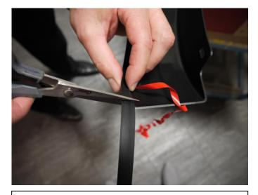
**STEP 3:** Trim rubber seal at end of each Fender Flare. Save extra rubber seal for install on opposite side Fender Flare and discard any excess once both sides are complete. **IMPORTANT NOTE:** Trim rubber seal.
