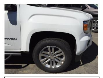
**STEP 4:** Clean the body areas where the Fender Flares will make contact. Ensure fenders are dry prior to install. Turning tires outward during install of each Fender Flare will ensure ease of install at bottom fixing points.
