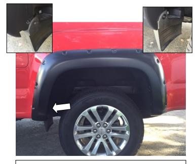
**STEP 12:** Place Fender Flare on the vehicle into the position of best fit, slide the bottom front end of Fender Flare between the existing mud flap deflector and wheel arch molding so that the slot in the Fender Flare is under the vacant hole in the mud flap. Using #15 Torx head screwdriver, loosely re-install the previously removed screw from front factory deflector.
