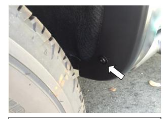
**STEP 9:** Loosely re-install previously removed factory screw through the slot in the Fender Flare at the bottom rear wheel arch using #15 Torx head screwdriver. Ensure Fender Flare is centered and in position of best fit on fender. Tighten all front fender fixing points to ensure a tight and secure fit. Ensure that the rubber seal is flush neatly against the vehicle body.
