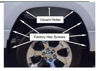
**STEP 8:** Hold Fender Flare towards vehicle in the position of best fit. Note (5) slots in Flare that correspond with factory installed hex screws, and the (3) that correspond with vacant holes in wheel arch. Remove (5) screws and retain for later re-installation.
