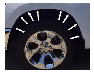
**STEP 5:** Hold Fender Flare towards vehicle in the position of best fit. Note the (8) slots in the flare that correspond with factory installed hex screws in the wheel arch. Remove these (8) and retain for later re-installation.
