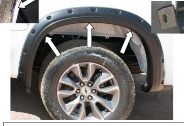
**STEP 17:** To secure the Fender Flare to the body, apply upward tension on Fender Flare to the vehicle fender when installing the black metal clips. Slide the clips over the Fender Flare and the inner wheel arch lip in the three locations shown. Position the clip so that the barb in the clip locates in the slot of the Fender Flare. Ensure all fixing points are tight and secure and that the extrusion is flush neatly against the vehicle body. Repeat install steps for the opposite side.
