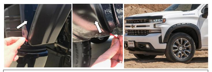
**STEP 9:** Starting at the front of the Fender Flare, carefully remove tape liner from extrusion a few inches at a time. Ensure extrusion is not tucking into flare and sits flush neatly against the fender body. Apply forward pressure to adhere the extrusion along the edge of entire length of Fender Flare once extrusion liner is removed. Ensure all fixing points are tight and secure and that the extrusion is flush neatly against the vehicle body. Repeat install steps for the opposite side.
