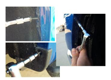
**STEP 6:** Remove three (3) 5.5mm bolts and two (2) 7mm bolt, retain for installation of Fender Flares.
