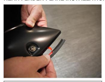
**STEP 10:** Attach the included rubber seal to the Fender Flares. Peel back 2" of the adhesive backing and position on the Fender Flare. Attach the seal to the Fender Flare, peeling back a few inches at a time. Attach rubber seal along all areas where the Fender Flare contacts the vehicle body.
