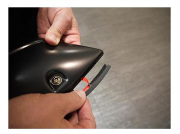
**STEP 1:** Attach the included rubber seal to the Fender Flares. Peel back 2" of the adhesive backing and position on the Fender Flare. Attach the seal to the Fender Flare, peeling back a few inches at a time. Attach rubber seal along all areas where the Fender Flare contacts the vehicle body.
