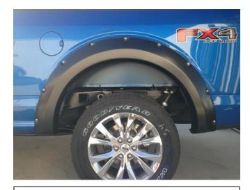
**STEP 15:** Repeat installation method for other side. Double check the front Fender Flares to make sure all bolts are tight and clips are securely fastened. Your installation is now complete. Do not use abrasive cleaners.
