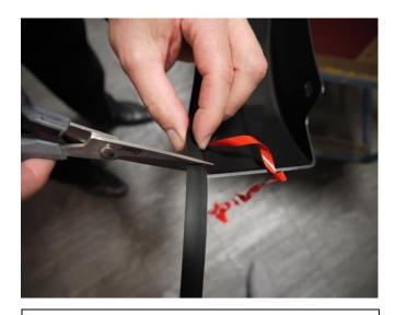
**STEP 12:** Trim any unnecessary extrusion and discard.
