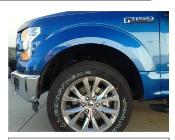
**STEP 4:** Clean the body areas where the Fender Flares will make contact. Use the supplied alcohol wipes.
