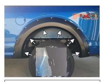
**STEP 14:** Place the Fender Flare onto the vehicle and fit into the correct position following the contours of the body. Use 6 of the U-style clips to secure the Fender Flare to the body. Make sure the barb in the clip securely attaches in the slot on the Fender Flare.
