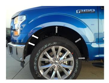
**STEP 5:** Locate three (3) 5.5mm bolts and two (2) 7mm bolt.
