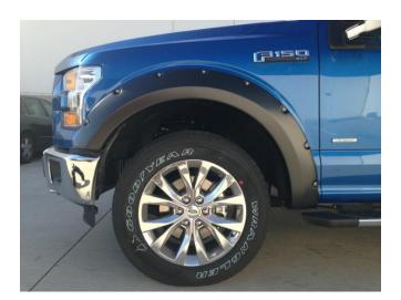
**STEP 9:** Repeat installation method for other side. Double check the front Fender Flares to make sure all bolts are tight and clips are securely fastened.
