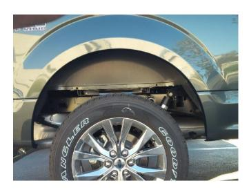
**STEP 13:** Clean the body areas where the Fender Flares will make contact. Use the supplied alcohol wipe.
