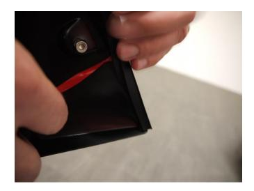
**STEP 11:** Pulling at right angles to the extrusion, remove the liner from the extrusion in small portions and apply thumb pressure to ensure that it adheres to the Fender Flares.
