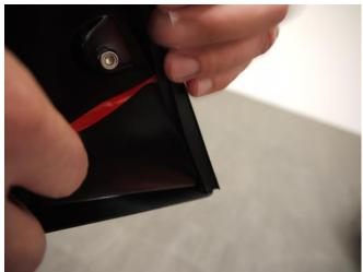
**STEP 2:** Pulling at right angles to the extrusion, remove the liner from the extrusion in small portions and apply thumb pressure to ensure that it adheres to the Fender Flares.
