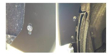
**STEP 8:** Reinstall the remaining 5.5mm bolt and two 7mm bolts.
