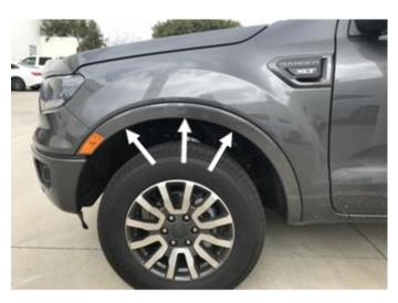
**STEP 6:** Using a Phillips head screwdriver remove factory wheel arch fasteners in the three shown locations. Install the screw plugs provided in the hardware kit into the shown locations.
