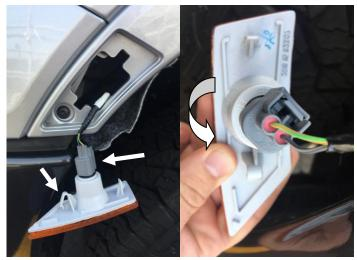
**STEP 4:** Removal of the turn signal is required for installation of front Fender Flares. Pull back the inner wheel well liner to locate the turn signal body and wiring. Remove the turn signal from the vehicle body by squeeze the lower tab on the back of the turn signal body. Carefully turn the wiring harness counterclockwise and remove the bulb-wiring harness from the turn signal body.
