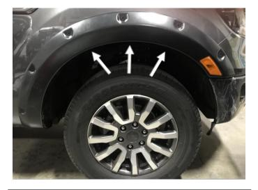
**STEP 7:** Attach the Fender Flare onto the vehicle into position of best fit. To secure the Fender Flare to the vehicle body, install the provided screws and washers into the screw plugs in the three shown locations.
