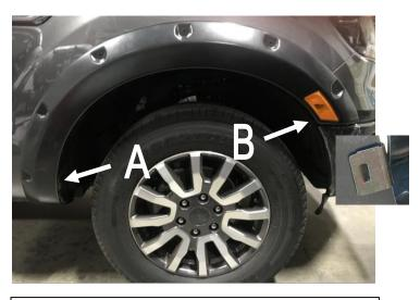
**STEP 8:** Apply upward tension on Fender Flare to the vehicle fender when installing the large U clip in location A and the small U clips in location B. Slide the clips over the Fender Flare and the inner wheel arch lip in the two locations shown. Position the clip so that the barb in the clip locates in the slot of the Fender Flare. Ensure all fixing points are tight and secure and that the rubber seal is flush neatly against the vehicle body. Repeat install steps for the opposite side.
