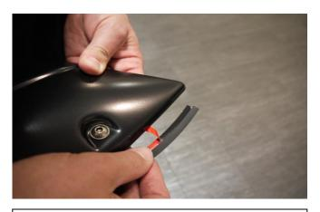
**STEP 9:** Attach the included rubber seal to the Fender Flares. Peel back 2" of the adhesive backing and position on the Fender Flare. Attach the seal to the Fender Flare, peeling back a few inches at a time. Ensure pressure is used to secure rubber seal to Fender Flare edge. Attach rubber seal along all areas the Fender Flare will make contact with the vehicle body. Trim excess rubber seal.
