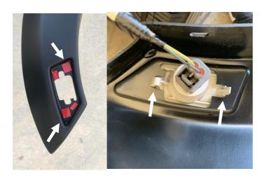
**STEP 5:** Apply the provided tape squares to the turn signal recess, cutting of the tapes will be required per image. Remove the tape liner, install the turn signal body into the recess in the front Fender Flares. Ensure the tabs in the back of the turn signal body snap into the Fender Flare recess pocket. Apply firm pressure across the turn signal once in place to achieve tape wet out. Reinstall the bulb-wiring harness to the turn signal body.
