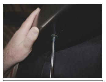
**STEP 7:** Place Fender Flare on the vehicle into the position of best fit so the slots in position **A**, **B** and **C** are over the holes in the front end of large clips. Ensure bottom rear slot in Fender Flare is located over the vacate hole in the factory mudguard. Apply upward tension on Fender Flare to the vehicle fender when Installing the screws and washers provided into the clips in position **A**, **B** and **C** using a Philips head screwdriver.
