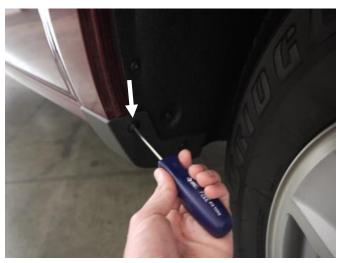
**STEP 5:** Using #15 Torx head screwdriver remove upper screw from the front factory mudguard. Maintain screws for re-install.
