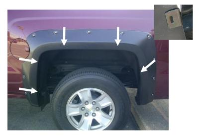
**STEP 13:** To secure the Fender Flare to the body, apply upward tension on Fender Flare to the vehicle fender when installing the black metal clips. Slide the clips over the Fender Flare and the inner wheel arch lip in the five locations shown. Position the clip so that the barb in the clip locates in the slot of the Fender Flare.
