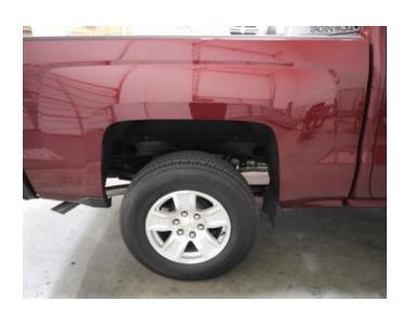
**STEP 11:** Clean the body areas where the Fender Flares will make contact. Ensure fenders are dry prior to install.
