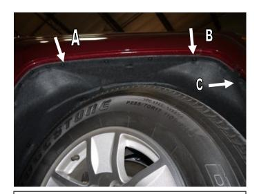
**STEP 4:** Dry fit the Fender Flare onto the vehicle in the position of best fit. Note where the slots in Fender Flare at positions **A**, **B and C** align with the existing screws in the vehicle wheel arch. Remove Fender Flare. Remove the existing vehicle screws in location **A**, **B and C** using #15 Torx head screwdriver. Maintain screws for re-install.
