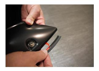
**STEP 9:** Attach the included rubber seal to the Fender Flares. Peel back 2" of the adhesive backing and position on the Fender Flare. Attach the seal to the Fender Flare, peeling back a few inches at a time. Ensure pressure is used to secure rubber seal to Fender Flare edge. Attach rubber seal along all areas where the Fender Flare contacts the vehicle body.
