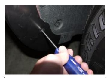
**STEP 8:** Re-install factory screw in the mudguard using #15 Torx head screwdriver through the slot in the Fender Flare.
