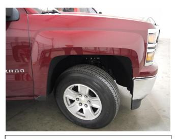
**STEP 3:** Clean the body areas where the Fender Flares will make contact. Ensure fenders are dry prior to install. Turn tires outward for Fender Flare installation.
