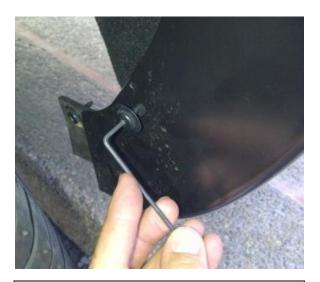
**STEP 14:** Using #15 Torx head screwdriver reinstall the upper screw from the rear factory mudguard through the slot in the Fender Flare. Ensure all fixing points are tight and secure and that the rubber seal is flush neatly against the vehicle body.
