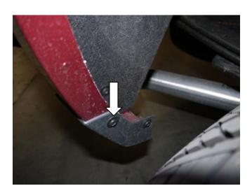
**STEP 12:** Using #15 Torx head screwdriver remove upper screw from the rear factory mudguard. Maintain screws for re-install.
