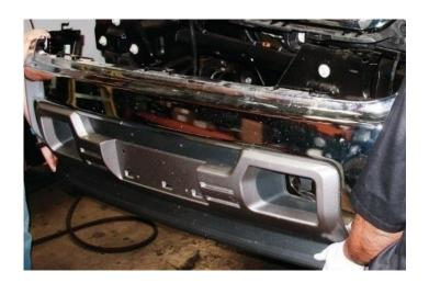
8: Remove six bolts holding on OEM frame flanges to frame with 15mm socket. Set bracket aside.
