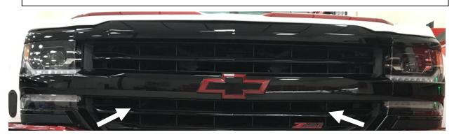
4: Unplug the OEM fog light and sensor wiring harness and place it up and out of the way.
