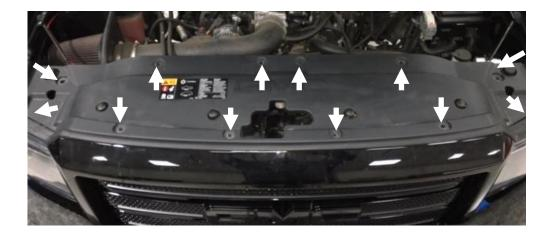
2: Remove four screws on top of grill with a 10mm socket.
