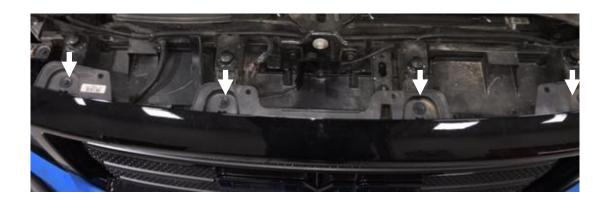
**3.** Remove the grill by pulling out on the bottom on both sides to release the tabs and then rotating the grill upwards. Set aside to re-install later.
