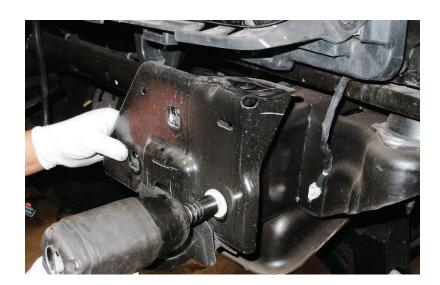
**9:** Remove two bolts holding on OEM tow hooks with 18mm socket and wrench. (both sides) Set tow hooks aside.
