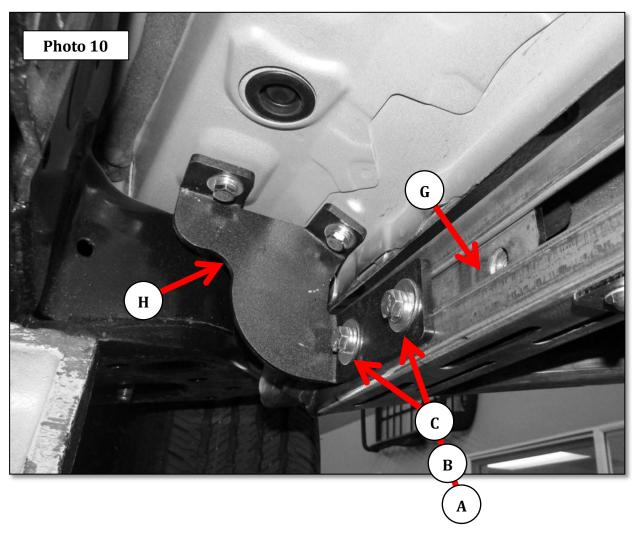
**Step-9** Align the running board with the vehicle and tighten all bracket and side step nuts and bolts,. Repeat the above steps to install the driver side brackets and Dominator D6 running board. Remember to check and retighten the nuts and bolts every six months.
