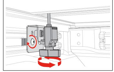
With the tailgate open and the front (cab) clamps secure, completely close the bed cover (A).
