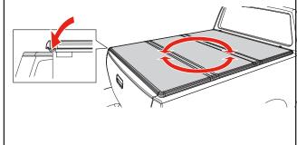
Carefully refold the bed cover (A) without shifting its position on the truck bed.
