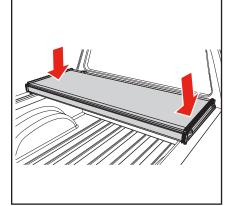
Unfold the bed cover (A) fully and adjust position over the truck bed for proper front (cab) and rear (tailgate) alignment. When positioned front and back, the tailgate seal should contact the tailgate with the first two fins.
