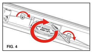
To make the final adjustment, loosen the striker bracket screws. Then move the bracket down by firmly pulling the cover to the truck rail and tailgate. Make sure that both sides match, then retighten the screws.
