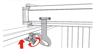
Close the tailgate and unfold the cover. Check that the cover is parallel and square with the truck bed and bed rails. If not parallel or square, open the cover and loosen the cab clamps to reposition the cover. Adjust and re-tighten both clamps.
