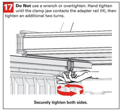
The tethers come installed on the bed cover hinge with a clamp at the other end. Install the clamp end by sliding the clamp onto the adapter rail (H). Make sure the clamp is positioned as far up onto the rail as possible. Firmly hand tighten the knobs. Install the tethers on both sides of the cover.
