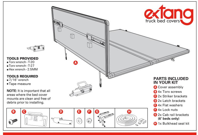
**IMPORTANT:** Please install the bulkhead seals (H) (for 5' & 6' beds) and the 2 cab rail brackets (G) (for 6' beds only) before proceeding. Separate installation sheets are found in the hardware bags.
