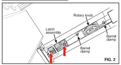
Rotate the rotary knob until you see the flat head screws. Tighten the two screws using the provided Torx T-20 wrench, (Fig. 3).
