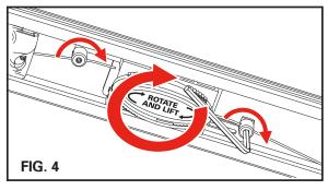
To make the final adjustment, loosen the striker bracket screws. Then move the bracket (C) down by firmly pushing the cover (A) or pulling the rear bow downward to the truck rail and tailgate. Make sure that both sides match, then retighten the screws.
