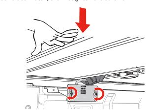
The tethers come installed on the bed cover hinge with a clamp at the other end. Install the clamp end by sliding the clamp onto the truck rail. Make sure the clamp is positioned as far up onto the rail as possible. Firmly hand tighten the knobs. Install the tethers on both sides of the cover.
