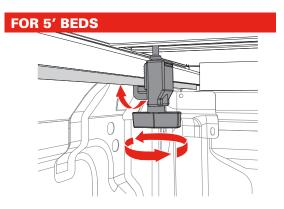
Hook the cab clamp under the truck bed rail metal flange. Tighten the knob until the jaw makes contact, then turn an additional two turns. Repeat on the opposite side of the truck bed.
