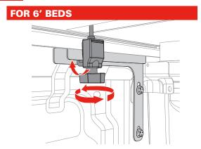
Hook the cab clamp under the installed cab rail brackets (G). Tighten the knob until the jaw makes contact, then turn an additional two turns. Repeat on the opposite side of the truck bed.
