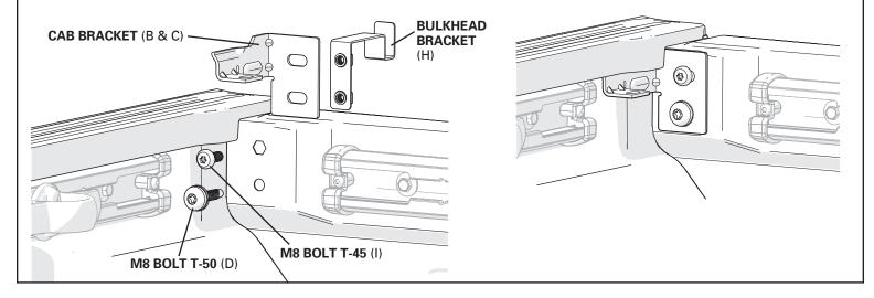
Before placing the cover (A) on the truck bed, remove both front clamp knobs. Leave the cab clamp rods in place.
