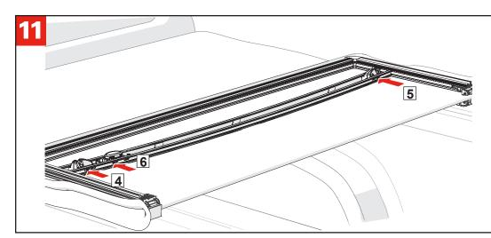
Fold the panel open and tighten the rear T-20 Torx screws in both the driver and passenger side latches and the actuator mechanism, shown below as 4, 5 & 6.
