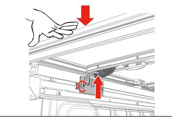
Adjustments and tightening of the latch assembly is required.
