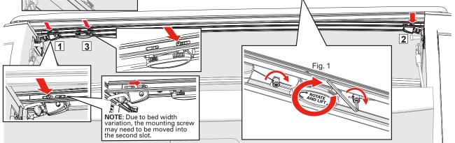
Double-check that the cover is secure and tight to the truck bed by gently lifting the corners to ensure the mechanisms are engaged.
