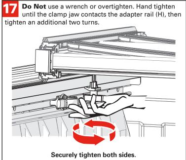
The tethers come installed looped over the bed cover bow with a clamp at the other end. Install the clamp end by sliding the clamp onto the adapter rail (H). Make sure the clamp is positioned as far up onto the rail as possible. Firmly hand tighten the knobs. Install the tethers on both sides of the cover.
