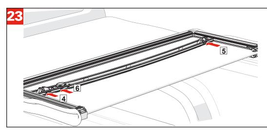
Fold the panel open and tighten the rear T-20 Torx screws in both the driver and passenger side latches and the actuator mechanism, shown to the left as 4, 5 & 6.
