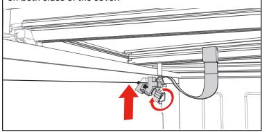
Close the tailgate and unfold the cover. Check that the cover is parallel and square with the truck bed and bed rails. If not parallel or square, open the cover and loosen the cab clamps to reposition the cover. Adjust and re-tighten both clamps.
