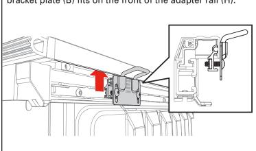
Close the cover (A) and align the striker bracket (B) with the bed cover latch. Push down on the cover while tightening the Torx screws (E).
