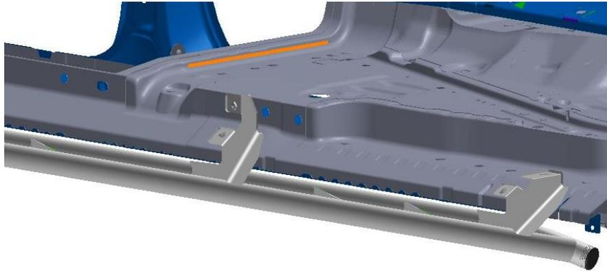
**Step 5:** Next, tighten the three lower bolts first, following with the three upper bolts.
