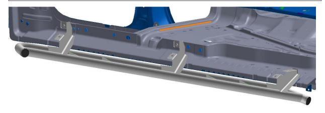
**Step 5:** Next, tighten the three lower bolts first, following with the three upper bolts.
