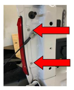
2. Fish the wire harness up from below the tailgate and out the tail light holes on each side of the truck.
