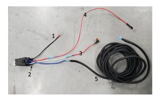
The power wire is a separate wire designed to power the freedom blade from battery. It uses a fuse tap style connector to tell the relay when to open or close, starting your Freedom Blade. This setup allows for maximum punch from the LED's. The power wire is packaged as a separate cable to allow easier wiring to the rear of the truck.
