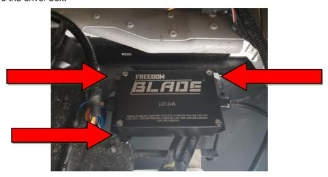
The Freedom Blade also comes with 3M automotive double sided sticky tape on the back of the driver box. If your truck has a suitable flat spot this can also be used for mounting. The 3M tape helps to reduce vibration.
