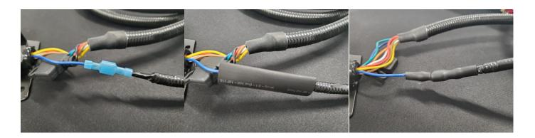
The power wire connects to the freedom blade using a spade terminal. Once connected, slide
