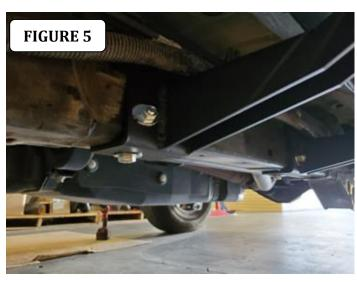
**Step-4** At the rear location, locate the threaded hole on the bottom of the frame and the slotted hole. Introduce a ½" bolt plate into the obround hole, use a vinyl gasket to prevent the bolt plate from falling into the frame rail. Secure the rear bracket to the bolt plate using (1) ½" flat, (1) ½" lock washer and (1) ½" hex nut. Secure the bottom hole using and (1) M12 hex bolt, (1) ½" flat washer and (1) ½" lock washer. Figure 7. Leave the bolt and nut loose for final adjustment.
