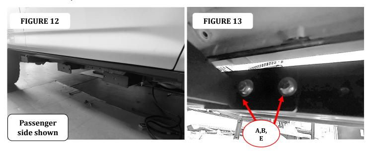
**Step-7** Align the Dominator running board with the vehicle and tighten all bolts securing the running board to the front, center and rear brackets. Repeat the above steps to install the driver side brackets and running board. Remember to check and retighten the nuts and bolts every six months.
