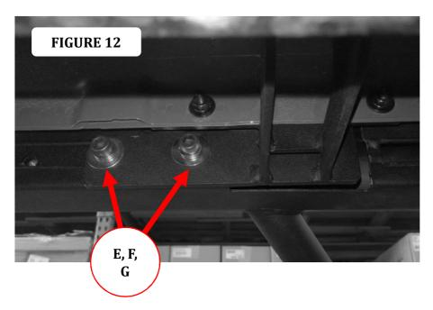
**Step-7** Align the Dominator running board with the vehicle and tighten all bolts securing the running board to the front, center and rear brackets. Repeat the above steps to install the passenger side brackets and running board. Remember to check and retighten the nuts and bolts every six months.
