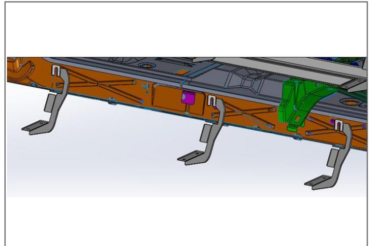
**Step 4.** Set running board along the top x3 brackets and center along the cab.
