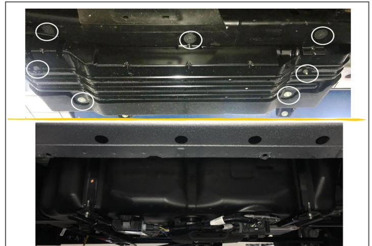
**Step 10.** Feed the short bracket (#5)x1 between the body and DEF tank, then align with lower rocker panel mount.
