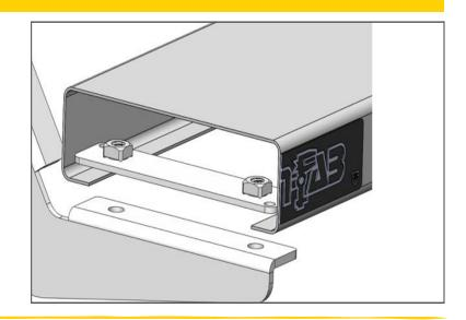
Step 9. For passenger side, remove the (x3) 13mm bolts, (x2) 10mm bolts and (x2) 10mm nuts that attach the Def tank cover. Remove and set aside.
