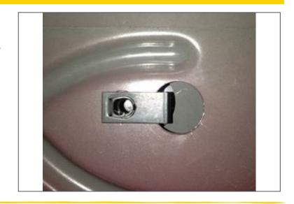
Step 3. Beginning with the driver side, install (#3)x2 mounting brackets using the supplied (#7)x4 M8x25mm hex bolt, (#8)x6 M8 fender washer and (#9)x4 M8 hex nut and loosely fasten.
