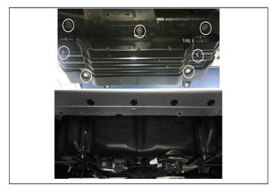
Step 10. Feed the short bracket (#5)x1 between the body and DEF tank, then align with lower rocker panel mount. Step 11. Use the supplied (#7)x4 M8x25mm hex bolt, (#8)x5 fender washer and (#9)x1 hex nut and tighten hardware to (15-20 ft/lbs).
