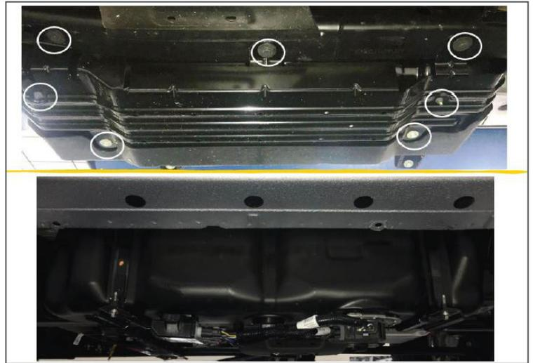
**Step 10.** Feed (#5)x1 upper bracket between the body and the Def tank until you locate the tab into the OE hole. The bracket will hang once placed correctly.
