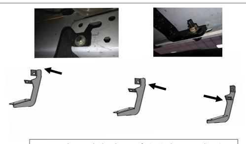
**NOTE:** Make sure the brackets are facing in the correct direction.
