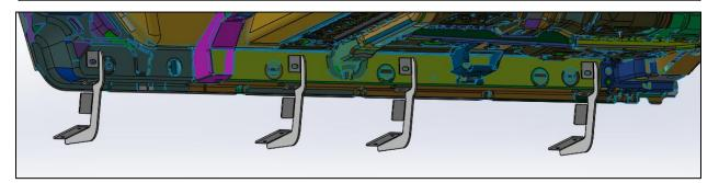
**<u>Step 4</u>**: Set running board along the top of all three brackets and center along the cab.
