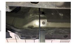
**Step 3:** Set running board along the top of the two brackets and center along the cab front/back.
