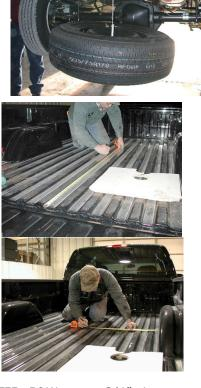
**TIP:** B&W uses a 3/4" piece of plywood as a drilling guide to prevent the hole saw from moving while drilling the 4" hole in the truck bed.
