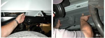
that protrudes from the center section must fit through the hole in the truck bed floor. Fasten the center section to the crossmembers using seven of the  $1/2" \times 1 1/2"$  bolts. Start these bolts through the holes in the crossmember and place a flat washer, a lock washer and nut on each bolt **DO NOT fully tighten at this time.**
