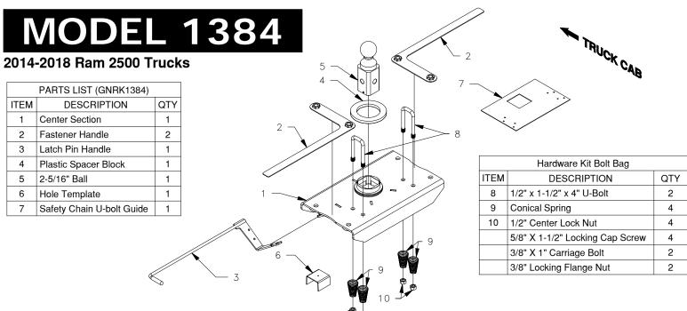
If you intend to use an 18K Companion 5th Wheel RV Hitch model 3000 in a 2014 or newer RAM ATTENTION: truck, please call us at 800-248-6564 for a kit that fills voids in the truck bed rib pattern. Using the model 3000 Companion on a 2014 or newer RAM without the supplemental kit could result in damage. RV Models 3400, 3405 and 3500 do not need a supplemental kit.
