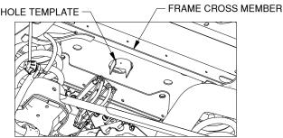
FIGURE A6: looking under truck bed towards cab.
