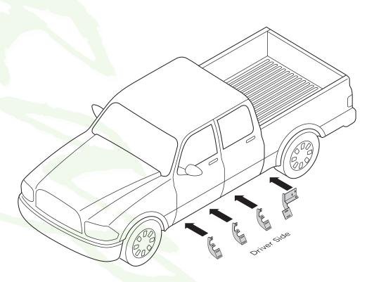
**4.** Existing mounting holes are located on the interior wall of the rocker panel. These mounting holes will be used per the following instruction.
