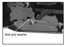
B. Insert bolt and washer through top of round hole in mounting bracket.
