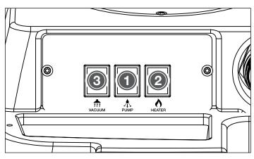
In order to avoid vapor locking the unit, the components should be switched on by following the procedure below after a cleaning tool is connected:
