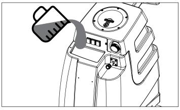
Lift the tank lid and, using a bucket, fill the solution tank via the large opening. For best results, use warm water. •
