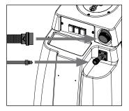
on the female fitting from the hose and slide onto the male fitting on the machine. Release to lock fittings together. •
