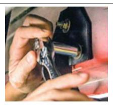
**Step 7.** After finial adjustment, tighten all three brackets at the main tube.
