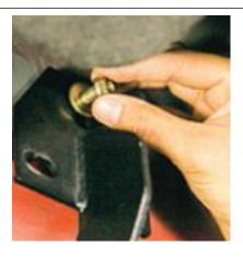
**Step 6.** Begin tightening nuts and bolts in an alternating pattern. Tighten to 20 (ft./lbs.) torque securing the steps to the vehicle.
