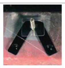
**Step 5.** Carefully hold step into place. Hand tighten the upper nut to bolt plate with washer. An assistant is recommended in the step. Insert and hand tighten lower bolt.
