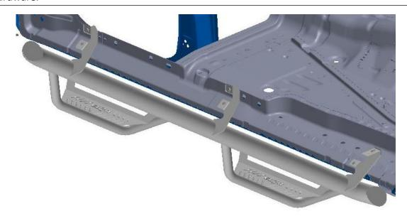
**Step 6:** Next, tighten the three lower bolts first following with the three upper bolts.
