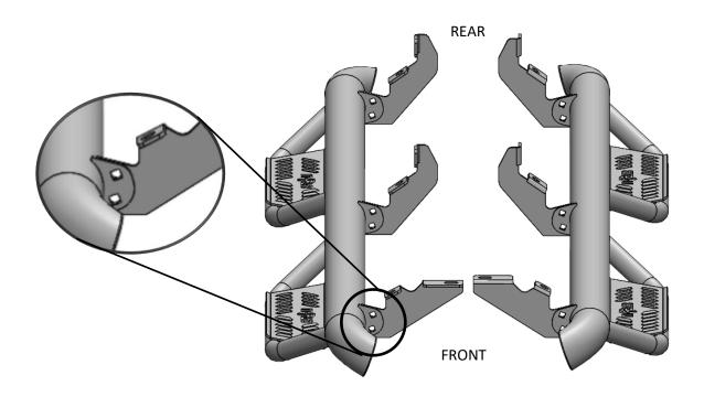
**STEP 3:** Remove any factory running boards or hardware and discard.
