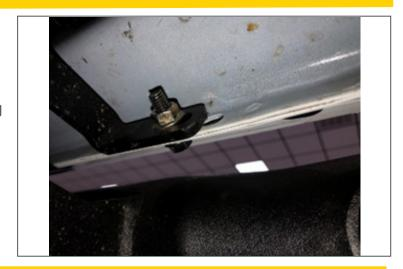
Step 7. Finish by tightening upper mounts. If M10x30mm bolts where used, torque to (**30 ft/lbs**) and (**20-25 ft/lbs**) for M8x30mm bolts.
