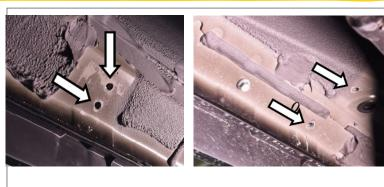
Step 3. Carefully place step into place aligning brackets with (x3) mounting location.
