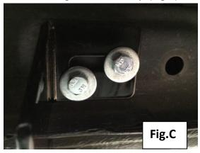
**Step 4:** Move to the front bracket and insert hardware finger tight and then to the rear bracket.
