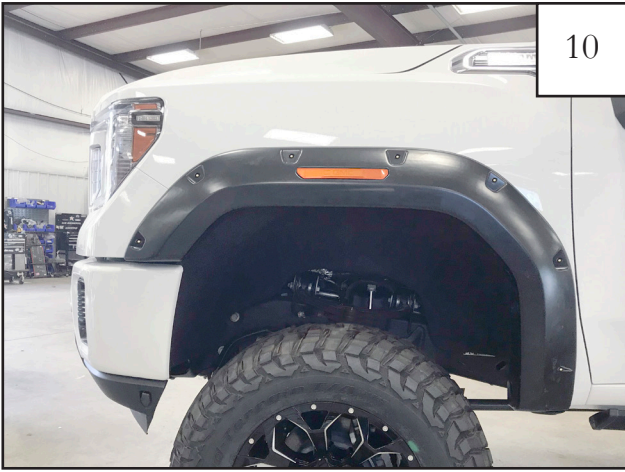
Completed front flare installation.
