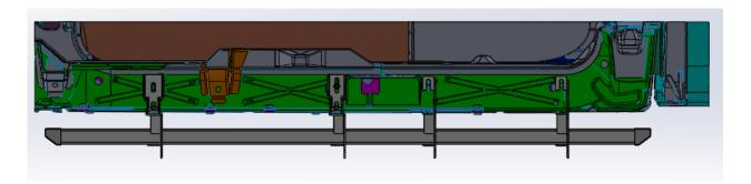
**Step 7:** Insert the supplied threaded brackets (x4) inside the running board lip over the top of each bracket.
