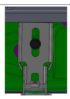
**Step 4:** Using the supplied M8x25mm hex bolts and washers begin hand tightening both upper and lower mounts to the rear two brackets.
