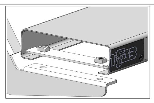
**Step 7:** After final adjustment, tighten all running board threaded mounts.
