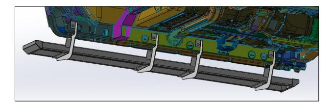
**Step 5:** Insert the supplied threaded brackets (x4) inside the running board lip over the top of each bracket.
