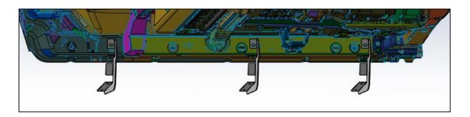
**<u>Step 4</u>**: Set running board along the top of all three brackets and center along the cab.
