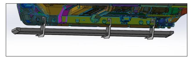
**<u>Step 5</u>**: Insert the supplied threaded brackets (x3) inside the running board lip over the top of each bracket.
