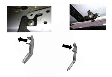
**NOTE:** Make sure the brackets are facing in the correct direction.
