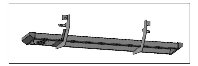
**Step 7:** Insert the supplied threaded brackets (x2) inside the running board lip over the top of each bracket.
