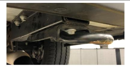
**<u>Step 2</u>**: Remove driver side and passenger side frame bolts and set aside. Save the bolts for the installation.
