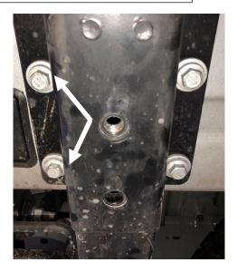
**<u>Step 3</u>**: Install the driver and passenger side-mounting bracket using the factory bolts removed from **Step 2**.
