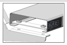
**<u>Step 6</u>**: After final adjustment, tighten all running board threaded mounts and frame bracket bolts.
